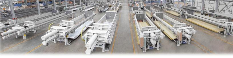
Modern mining requires efficient, cost-effective and environmentally friendly technologies for fine solids dewatering. A filter press, schematically shown below, utilizes the pressure difference provided by the feed pump and pressurized media to achieve solid-liquid separation and has been gaining popularity in the mining industry for both tailings as well as ore concentrate fines dewatering.
